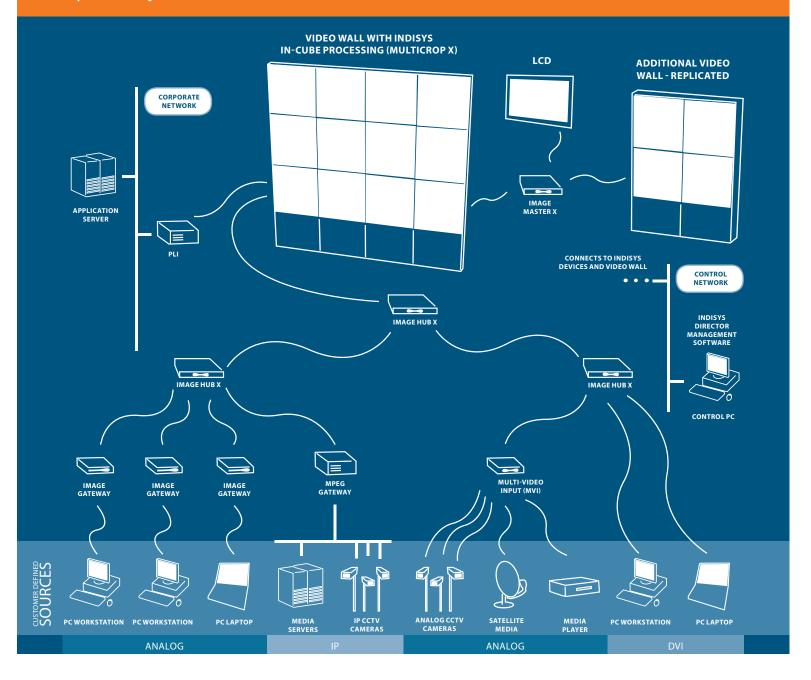
The Indisys solution uses a network architecture to create a visual network delivering the customer's information on video walls and external displays with maximum flexibility, reliability and control. The system can be described in four parts defined below:
